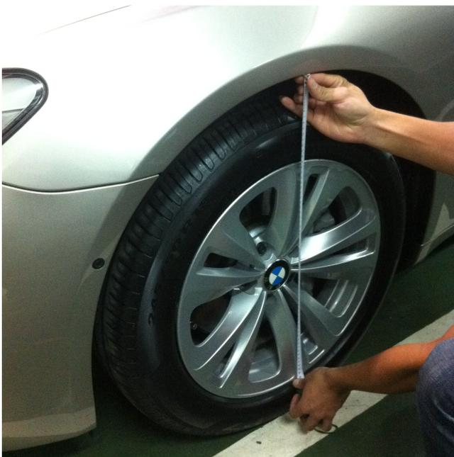
Measure the distance between lowest point of the rim and the nearest vertical point of the shroud.
