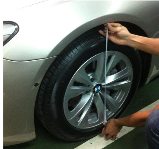
Measure the distance between lowest point of the rim and the nearest vertical point of the shroud.
